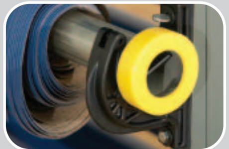
Yellow collar holds cover roller captive and eliminates finger pinch points.
