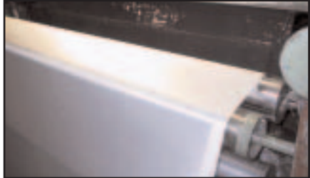
A knife and roller press spread the polymer into the core for complete saturation.
