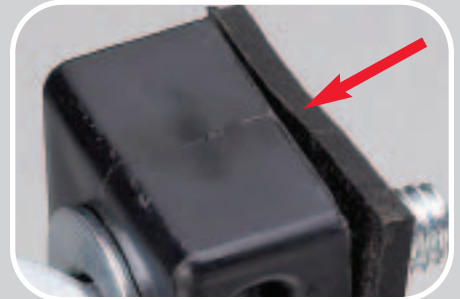
Roller brackets are mounted with 1/8" thick, shock absorbing rubber pads.
