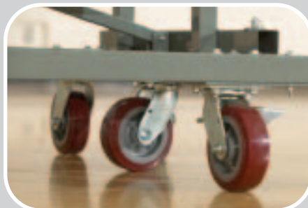
1 of 3 casters at each end is offset to spread load over larger area and to better protect the floor.
